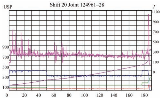
Figure 2. Example of record of the parameters of continuous flash-butt welding process of rails on stationary rail welding machine K1000
