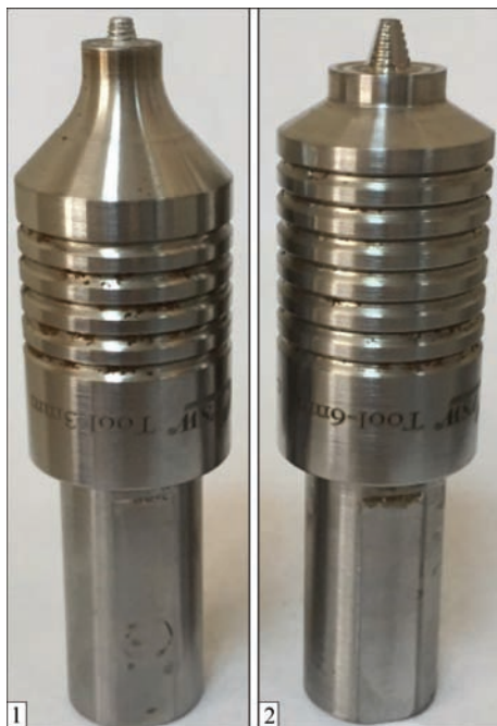
Figure 2. The FSW stirring tools used in this study (1 — pin length is 2.8 mm and shoulder diameter is 10 mm; 2 — pin length is 6.0 mm and shoulder diameter is 15 mm) [38]
