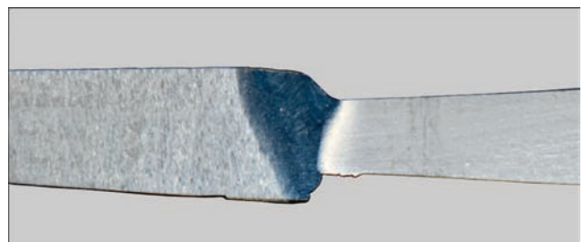
Figure 11. General view of welded joint of the blade repair shop bay
