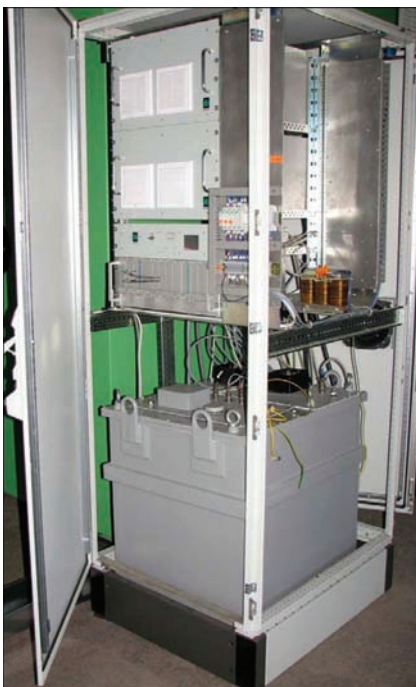
Figure 5. Appearance of inverter high-voltage power source
