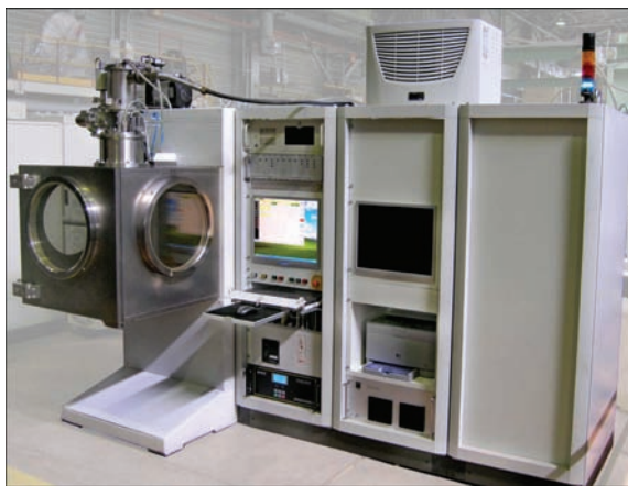
Figure 1. Appearance of small-sized electron beam installation. Additional flexibility is provided by welding manipulator with an inclined axis of rotation. It allows inclining the rotation axis of the faceplate in the range from 30^\circ to +90^\circ (from vertical), which provides electron beam welding of intricate concentric sections of aircraft engines or aircraft assemblies with a varying geometry (Figure 4).
