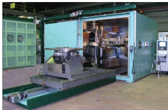
Figure 2. Appearance of medium-sized installation with a mobile intra-chamber welding gun and wheel-out working table
