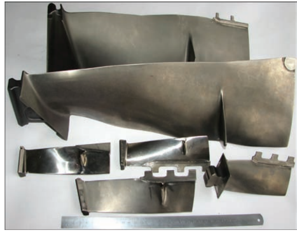
Figure 10. Examples of fan blades, repaired by electron beam produced by a single-pass EBW, and a smooth transition from the surface of the insert to the base metal is provided both by a moderate concentration of the electron beam and also by a sufficient amount of additional metal due to the applied design of welded joint with an overhanging flange. This allows obtaining a smooth transition of metal from the insert to the surfaces of the blade airfoil, both in the places with a sufficiently large thickness of the airfoil, as well as in the thinnest places adjacent to the very edge of the airfoil.
