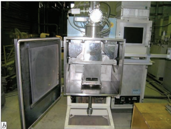
Figure 13. Scheme (a) and industrial model (b) of installation for additive manufacturing using metallic powder materials, where 1 — vacuum chamber; 2 — electron beam gun; 3 — hopper; 4 — table; 5 — rack; 6 — shaft; 7 — pallet; 8 — product; 9 — powder the chamber, as well as the development of appropriate software for realizing the additive manufacturing.
