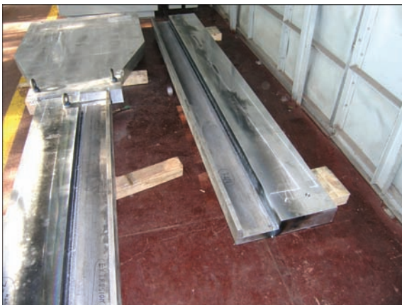
Figure 9. Appearance of welded thick-sheet aircraft structures of high-strength aluminum alloys
