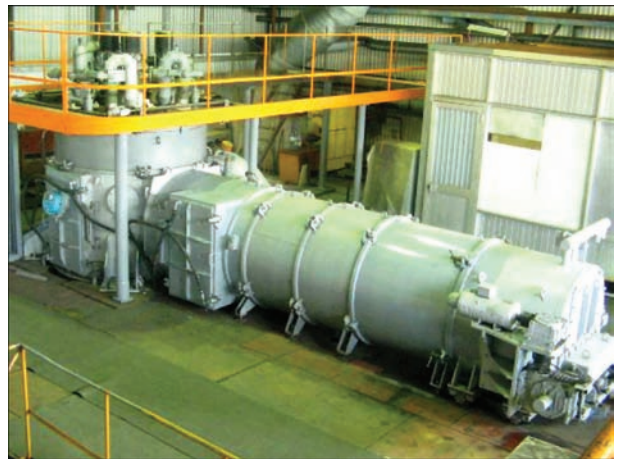
Figure 9. Appearance of commercial electron beam unit UE5812 of up to 840 mm diameter and design equipment for their commercial realizing (Figures 8, 9).
