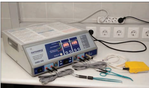
Figure 24. Apparatus EKVZ -300 Patonmed for welding of live tissues
