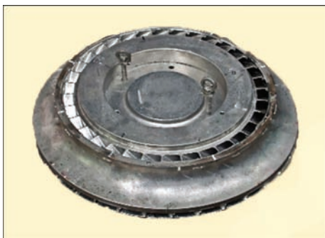
Figure 19. Gas turbine engine compressor centrifugal wheel, manufactured by applying the new brazing alloy
