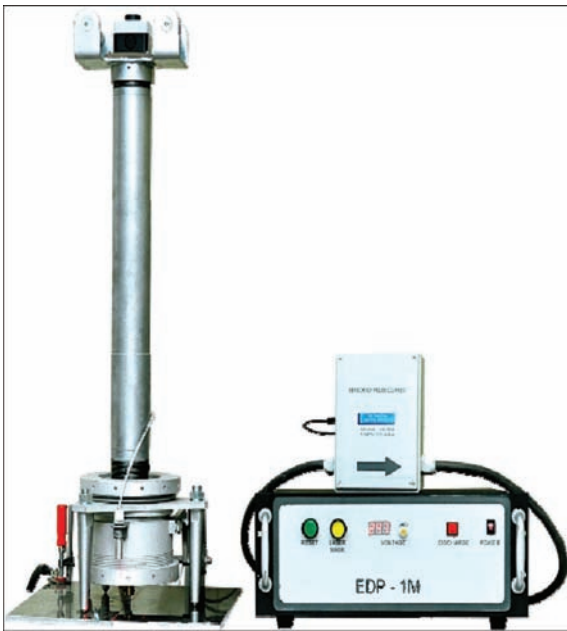
Figure 17. Manual tool and mobile power source for EDT
