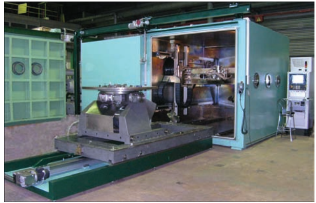
Figure 5. Typical medium-sized chamber with a mobile gun and wheeled-out table
