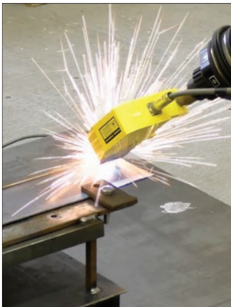
Figure 14. Welding robot with a technical vision system [7]
