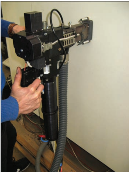
Figure 4. Semi-automatic manual laser tool
