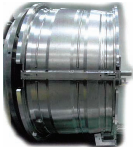
Figure 6. Welded billet of aircraft engine section of titanium alloy VT-6
