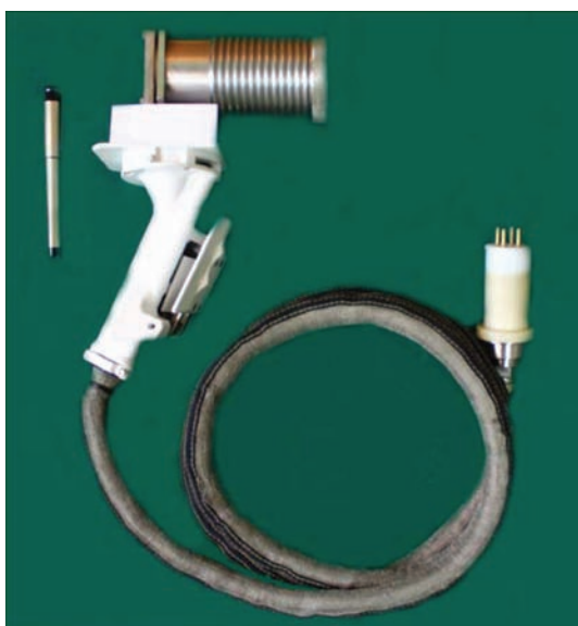
Figure 7. Manual electron beam gun with a high-voltage connector
