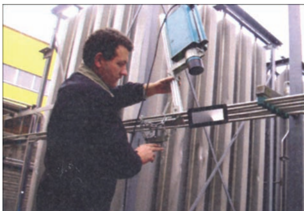
Figure 20. Portable digital X-ray-TV equipment arranged on object
