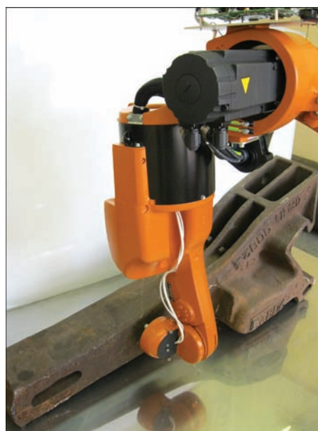
Figure 21. Robot with technical vision system for nondestructive testing of intricate geometry products [20]
