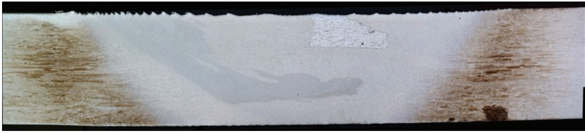
Figure 11. Structure of a weld in case of location of a rod of EN AC 43200 on retreating side (as in Figure 9, b ). Welding parameters: \omega = 450 \text{ min}^{-1} , V = 224 \text{ mm/min} . Keller etching
