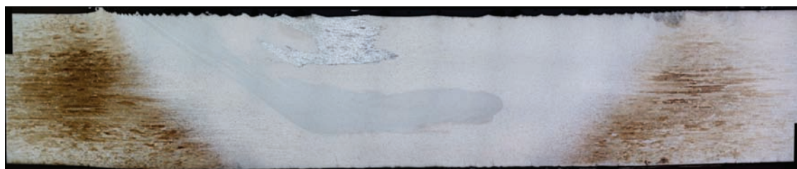
Figure 10. Structure of FSW weld in case of location EN AC 43200 rod (A) on the advancing side (as in Figure 9, a). Welding parameters: \omega = 450 \text{ min}^{-1} , V = 224 \text{ mm/min} . Triflute tool. Keller etching
