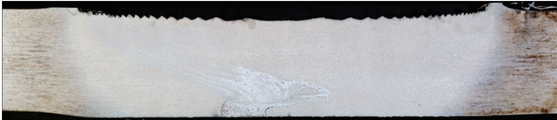
Figure 12. Structure of a weld in case of location of a rod of EN AC 43200 in the root on the advancing side (as in Figure 9, c ). Welding parameters: \omega = 450 \text{ min}^{-1} , V_{zg} = 224 \text{ mm/min} . Keller etching
