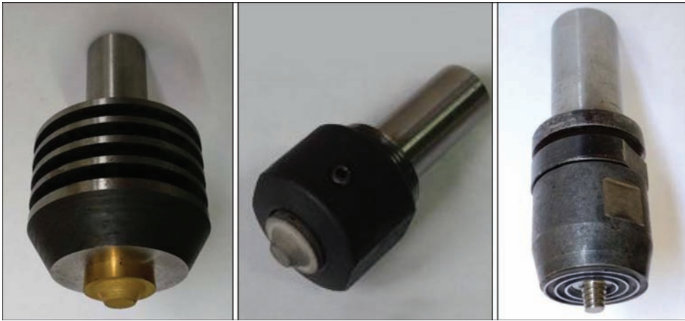
Figure 4. Examples of tools produced by the methods of powder metallurgy and 3D-printing
