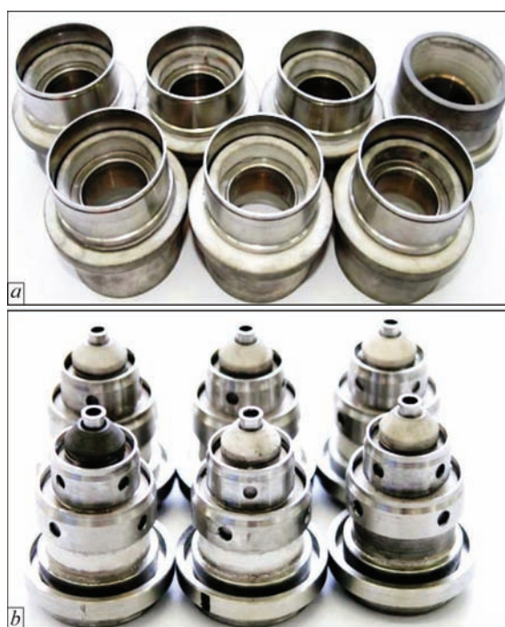
Figure 8. Metal-ceramic assemblies produced by brazing without ceramics metallization
