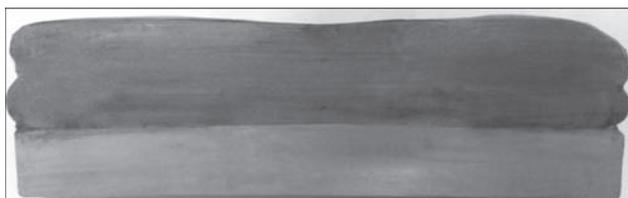
Figure 3. Macrosection of bimetal billet from experiment 45M
