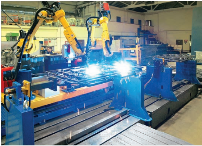
Robotic complex for welding of container walls
