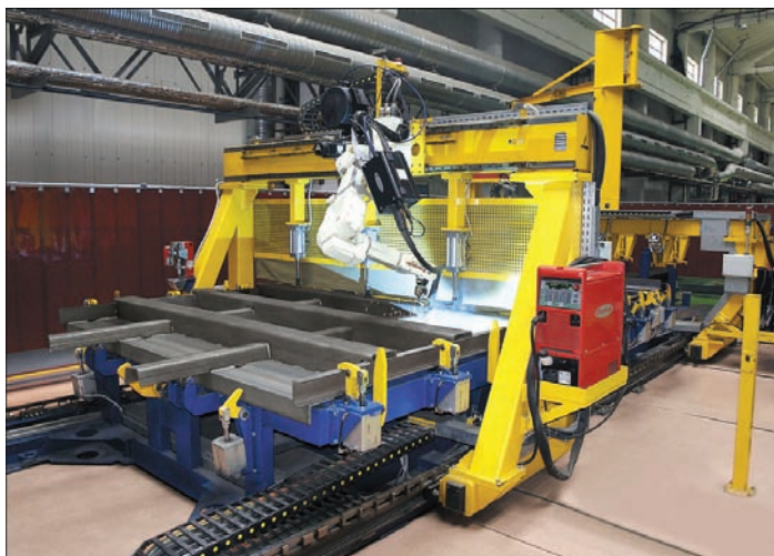
Robotic complex for welding of transverse carriage beams
