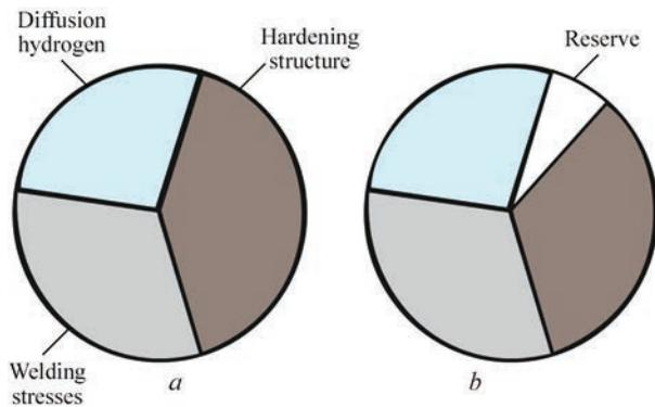
**Figure 7.** Factors, promoting delayed fracture of welded joints (*a* — critical state; *b* — state with reserve of cracking resistance)
