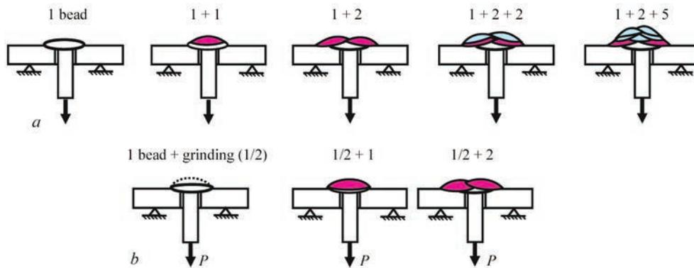
**Figure 2.** Technological schemes of welding of test joints: *a* — welding with simple beads; *b* — welding with first bead grinding
