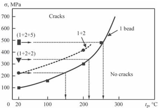
**Figure 5.** Comparison of the test results in welding with reheating without preheating ( $t_p = 20$  °C) and welding with preheating ( $t_p$  — temperature of preheating)
