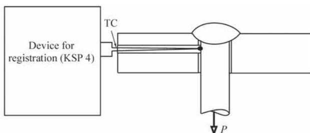
**Figure 1.** Scheme of measurement of temperature in Implant sample
