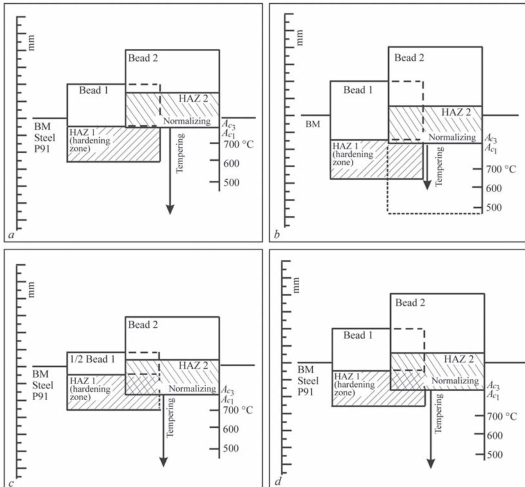
**Figure 6.** Distribution of temperatures in near-weld zone in performance of two beads (*a, b* — conventional welding: *a* —  $I_w = 100$  A,  $q/v = 8.3$  kJ/cm; *b* —  $I_w = 160$  A,  $q/v = 11.38$  kJ/cm; *c* — welding with first bead grinding,  $I_w = 100$  A; *d* — welding with simple bead, first bead is made on current  $I_w = 100$  A; second — 160 A)
