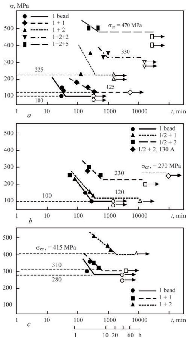
**Figure 4.** Results of tests: *a* — welding without heating with simple bead; *b* — welding without heating with grinding of the first bead for 1/2 of its thickness; *c* — welding with 200 °C preheating (dark and light marks — joints with and without fractures)
