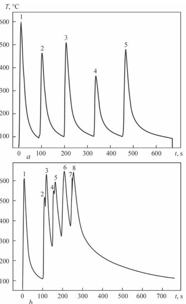
**Figure 3.** Thermal cycles in place of TC welding to sample in performance of test joints on 1 + 2 + 2 beads scheme (*a*) and on 1 + 2 + 5 beads scheme using principle of «transverse hill» welding (*b*)
