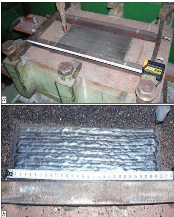
Figures 5. Appearance of 3 mm thick steel sheet prepared for surfacing (a) and a fragment of deposited sheet (b)
