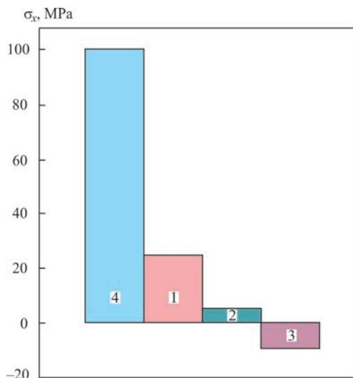
**Figure 4.** Peak values of stresses  $\sigma_x$  in weld center of welded plate of alloy AMg6 of  $400 \times 100 \times 2$  mm size, where numbers of columns 1–3 of values  $\sigma_x$  correspond to numbers of curves in Figure 3 (column 4 —  $\sigma_x$  without EDT)
