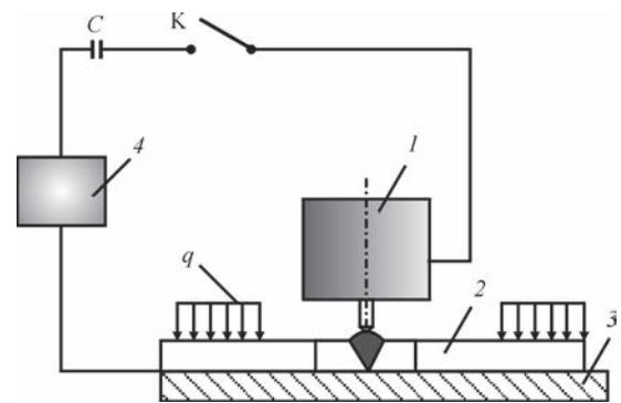
**Figure 2.** EDT of specimens of welded joints of alloy AMg6 at «rigid» fixation: C — capacitive energy storage; K — power switch;  $q$  — fixing load; 1 — ED; 2 — specimen; 3 — assembly plate; 4 — Hall sensor
