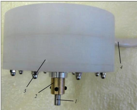
**Figure 1.** Electrode device for EDT (see designations in the text) protective casing 3, which contains the device, providing the effect of electric pulsed and dynamic components of EDT on the welded joint. Power cable 4 provided connection of ED to SPEC.
