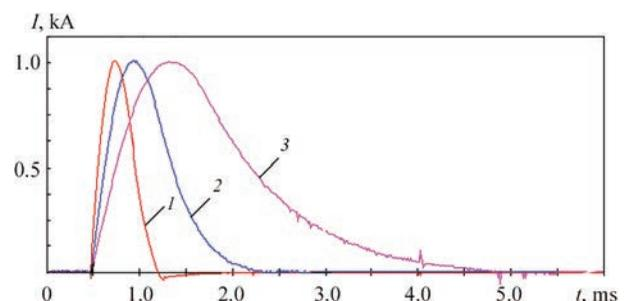
**Figure 3.** Time distribution of pulsed current  $I$  of equal amplitude at EDT of welded plates of alloy AMg6 of 400×100×2 mm sizes, where numbers of curves correspond to numbers of Table lines
