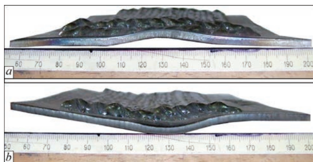
Figure 4. Appearance of deformed transverse edge of plate after surfacing of two layers with wire PP-Np-25Kh5FMS at fixation without a gap (a) and with a gap (b)
