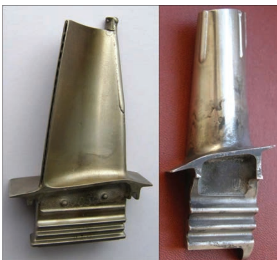
Figure 9. Appearance of single-crystal blades from ZhS32 alloy with repair welds
