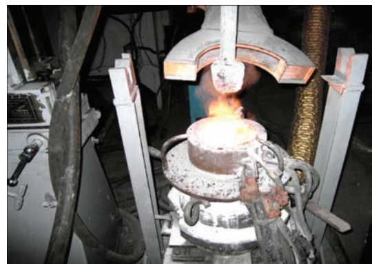
Figure 4. Stage of start of CCM work at removed from slag pool water-cooled electrode with graphite tip
