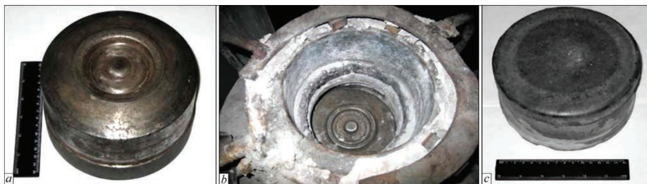
Figure 5. Press die of 170 mm diameter and 80 mm height of steel 5KhNM: a — before surfacing; b — in mold before surfacing; c — after surfacing
