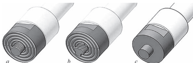
Figure 2. Tools for friction stir welding: a — type C; b — T; c — S
