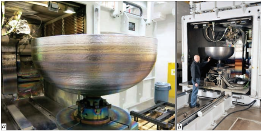
Fig re 1 Rocket fuel tank (a) and electron beam chamber for 3D printing (b) [5]
