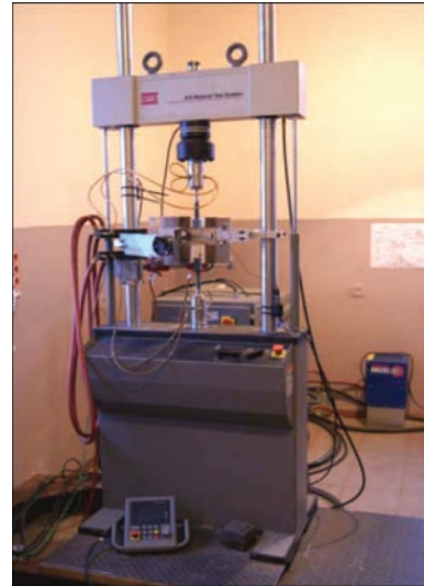
Figure 7. Appearance of servohydraulic machine MTS-810 for high-temperature tests of difficult-to-weld nickel high-temperature alloys
