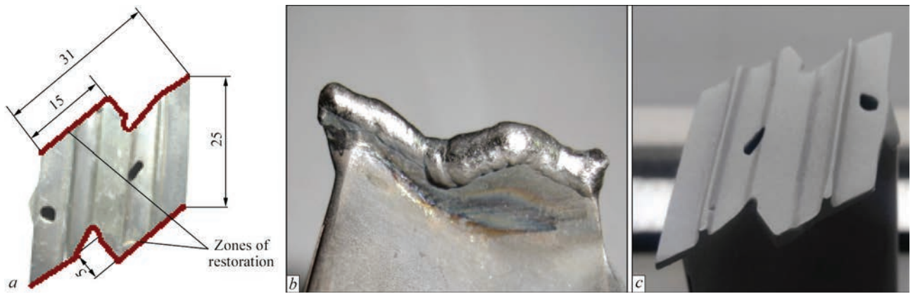
Figure 1. Appearance of pilot turbine blade of nickel high-temperature alloy ZhS6U restored by microplasma powder surfacing of ZhS6K alloy: a — characteristics of repair zone; b — appearance of deposited flange platform with Z-profile; c — appearance of restored flange platform after machining and penetrant testing
