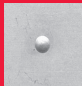
Plasma spot welding of 1 + 1 mm sheets
