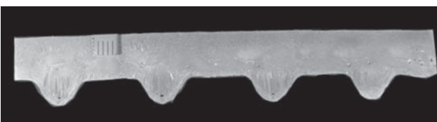
Figure 18. Longitudinal section of butt joint of 8 mm thickness — humps and porosity
