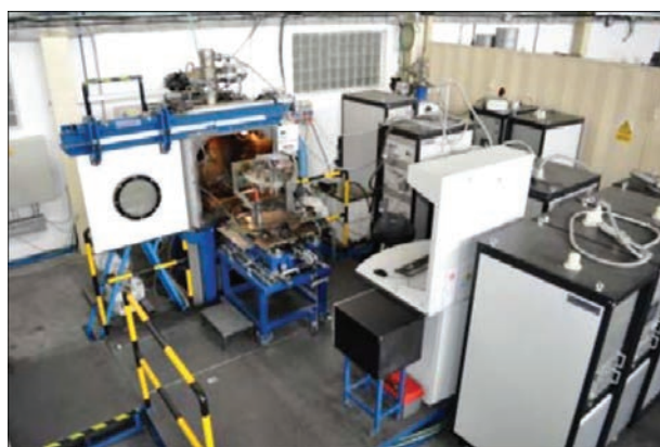
Figure 1. Workplace of electron-beam complex PZ EZ 4
