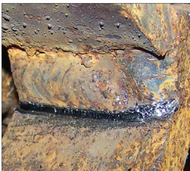
Figure 2. Appearance of weld zone of a tee welded joint of 15KhSND steel after testing by 2 \cdot 10^6 cycles, corrosion testing for 1200 h in the hydrostat and strengthening by HFMP technology
