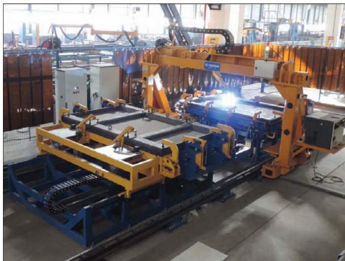
Robotic complex for welding of rear tail boards of dump trucks
