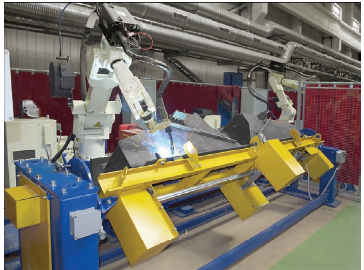
Robotic complex for welding of heating boilers
