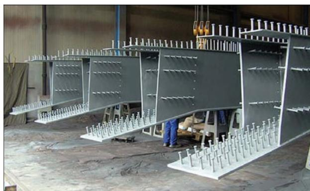
**Figure 13.** Shear studs in civil engineering (source: Schöler + Bolte)
