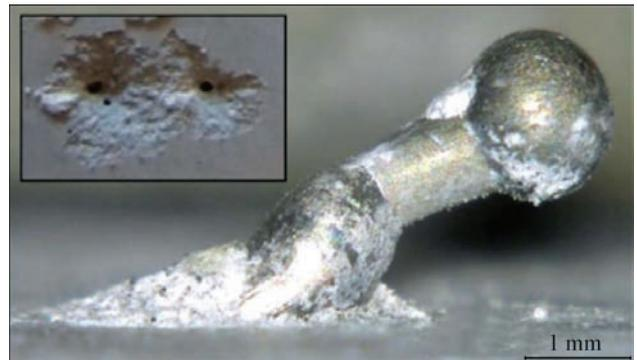
**Figure 16.** Die cutting failure of concrete-pin connection
