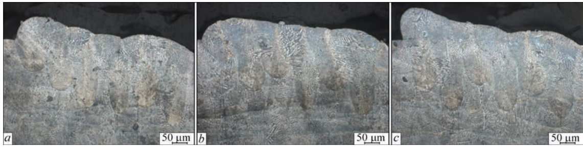
Figure 3. Microstructure of single layer at a laser power of 200 W and scanning speed: a — 800 mm/s ( E = 50 \text{ J/mm}^3 ); b — 750 mm/s ( E = 53 \text{ J/mm}^3 ); c — 700 mm/s ( E = 57 \text{ J/mm}^3 )
