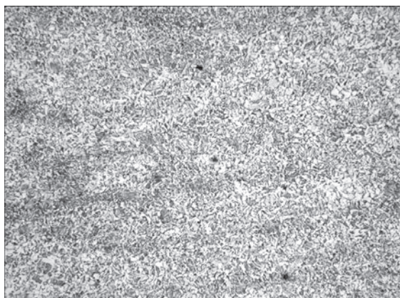
Figure 13. Microstructure ( \times 200 ) of the area of complete and partial recrystallization on the pipe side
