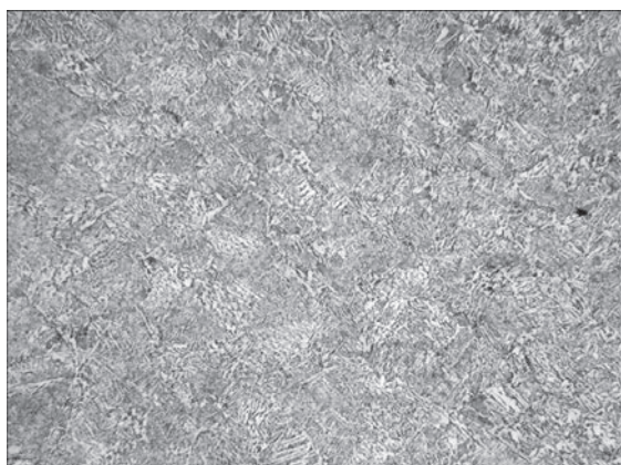
Figure 12. Microstructure ( \times 200 ) of the overheating area on the pipe side
