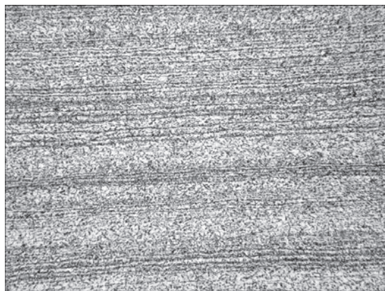
Figure 14. Microstructure ( \times 200 ) of base metal of the pipe
