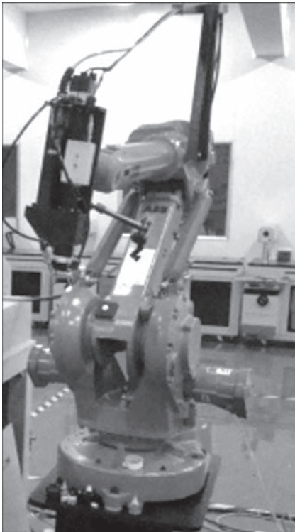
Figure 7. Appearance of robotic laboratory bench for laser arc welding with laser focus oscillations
