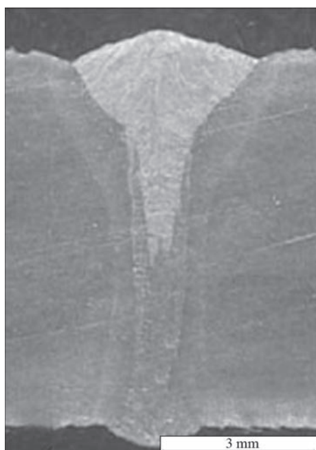
Figure 3. Absence of a uniform distribution of the electrode wire metal along the weld depth during laser-MIG welding of steels of large (over 8 mm) thicknesses on the example of welding SSAB Domex 420MS steel (standard EN 10149-2) [8]
