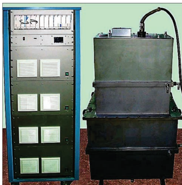
Figure 4. High-voltage source with control cabinet
