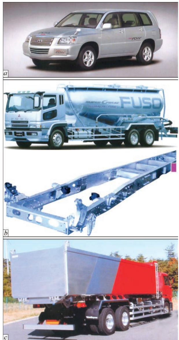
Figure 6. Examples of aluminium alloy application in trucks: a — Toyota FCHV; b — superlight truck FU with aluminium frames; c — aluminium alloy body of a dump truck
