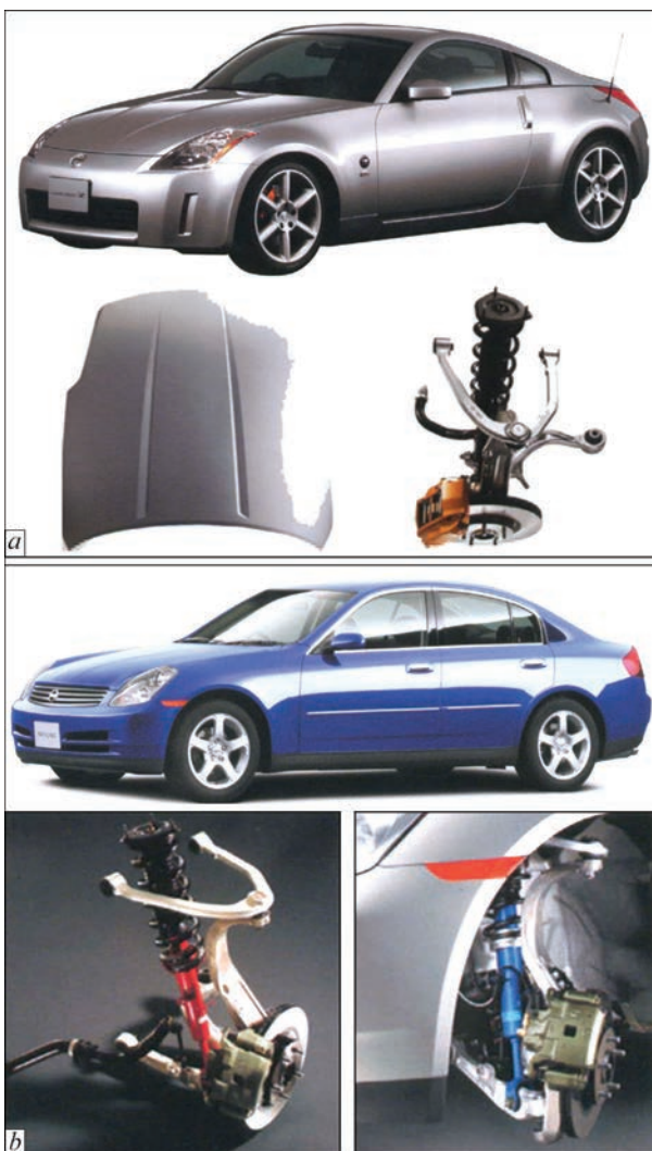
Figure 5. Examples of aluminium alloy application in passenger cars: a — Ferrari Z33; b — Skyline V35
