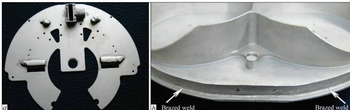
Figure 2. Appearance of thin-walled aluminium waveguide ( a ), brazed weld along the perimeter of the structure ( b )
