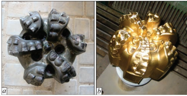
Figure 9. Matrix drill bit of 215.9 mm diameter for surface drilling during oil and gas production before (a) and after repair (b)
