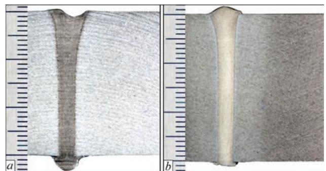
Figure 5. Cross-sections of joints of plates of 1570 alloy welded at a speed of 2.8 (a) and 16.8 mm/s (b)
