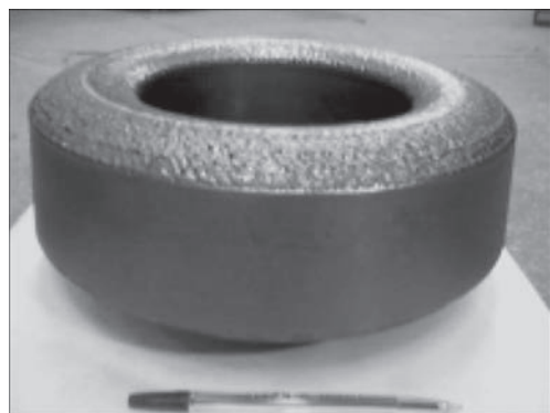
Figure 3. Appearance of the tuyere head of a blast furnace, surfaced by electron beam method [27]
