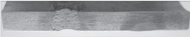
Figure 3. Macrostructure of welded joint of specimen-simulator of pipe elements of HPH spiral (position joints), produced using automatic orbital helium arc welding by the method of autopressing, where on the left a weld is shown formed in a one pass by automatic orbital helium arc welding, and on the right the weld is shown formed by automatic orbital argon arc welding applying the same method
