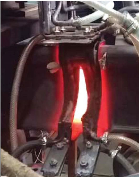
Figure 7. Heating of welded butt joint of R65 rail by a test split inductor without magnetic circuit
