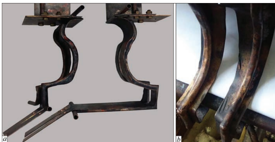
Figure 5. Laboratory test sample of a split inductor without magnetic circuits
