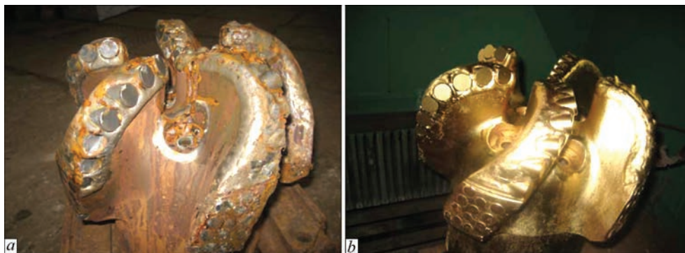
Figure 7. Integral steel drill bit of 295.3 mm diameter of «Volgaburmash» (Russia): before ( a ) and after repair ( b )
