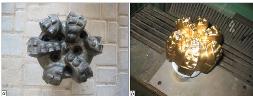
Figure 6. Matrix drill bit of 215.9 mm diameter: a — before repair; b — after repair
