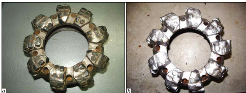
Figure 8. Integral drill head of 212.7 mm diameter of «Burinteks» (Russia): before ( a ) and after repair ( b )
