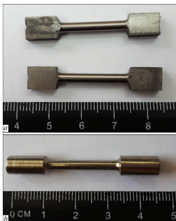
Figure 1. Appearance of intermetallic specimen, made for mechanical tests: a — thickness 3; b — 10 mm
