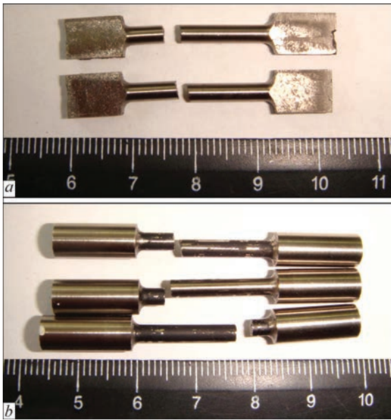
Figure 2. Intermetallic specimens after tensile test: a — thickness 3; b — 10 mm
