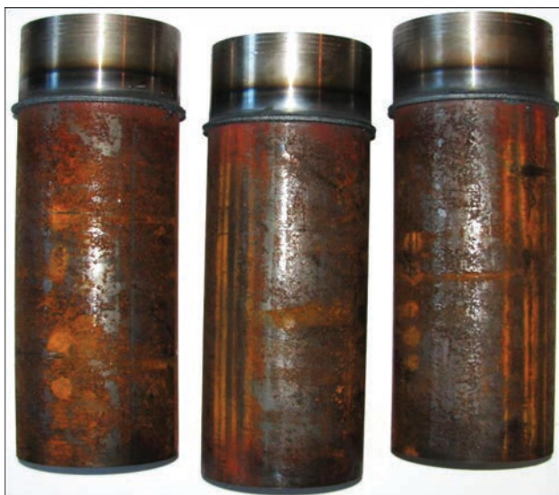
Figure 2. Welded joint of tubular parts of 102×6 mm
