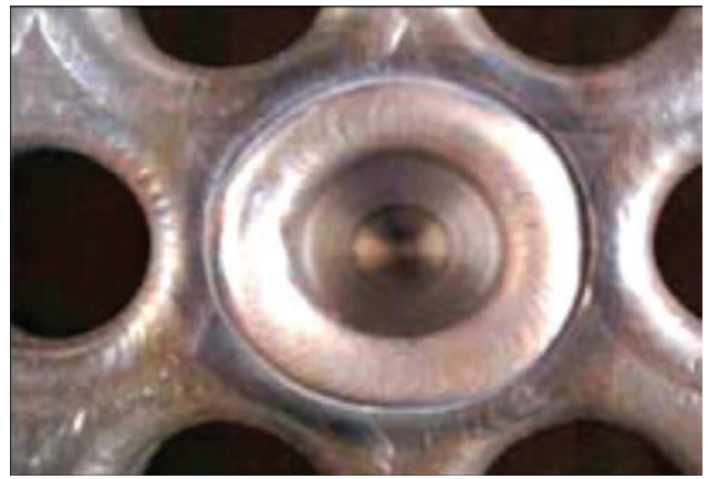
Figure 3. Plug installed using argon-arc welding [18]
