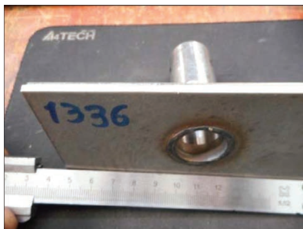
Figure 4. Plate-tube type joint after laser welding
