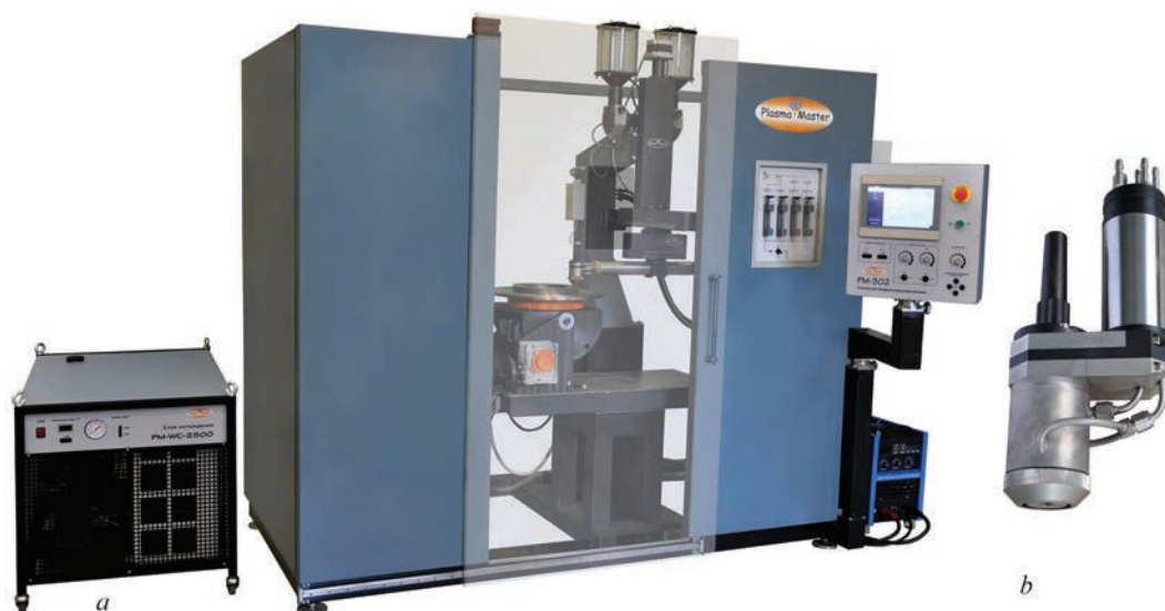
Figure 10. Equipment for PTA surfacing with composite alloys with separate powder feed: a — PM-302 unit; b — PP-6-04 PTA torch
