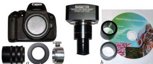
Figure 3. Photography equipment used for modernization of the microscope MIM-7: camera Canon 650D with adapters made for it ( a ); video eyepiece SIGETA MCMOS 3100 with set adapters and SW Topview ( b )
