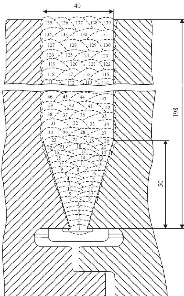
**Figure 1.** Scheme of automatic welding of a rotor model
