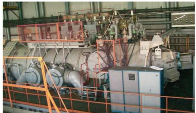
All-purpose electron beam installation UE5810
