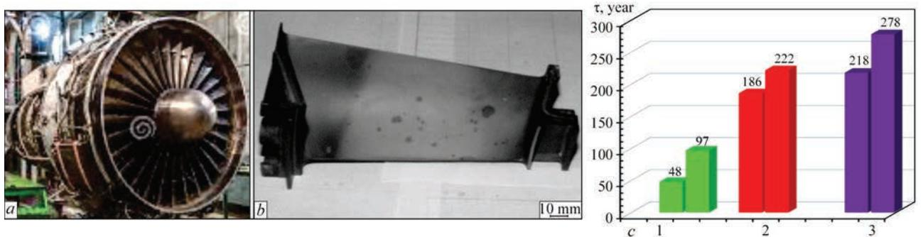
**Figure 12.** Gas-turbine engine (a), blade (b), long-term strength of butt similar brazed joints Ni<sub>3</sub>Al+Ni<sub>3</sub>Al produced using multicomponent nickel brazing filler metal without heat treatment (1), with heat treatment (2) and dissimilar joints Ni<sub>3</sub>Al+ZrS6U with heat treatment
