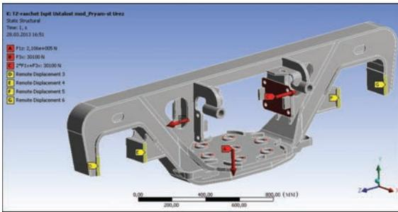
**Figure 1.** Vertical load  $F_{1z} = 210.6$  kN (A), uniformly distributed over the area of spring suspension on the support surface of the central spring suspension, and the wedge span force  $F_{3x} = 30.1$  kN (B), which are applied to the vertical posts of the central spring hole
