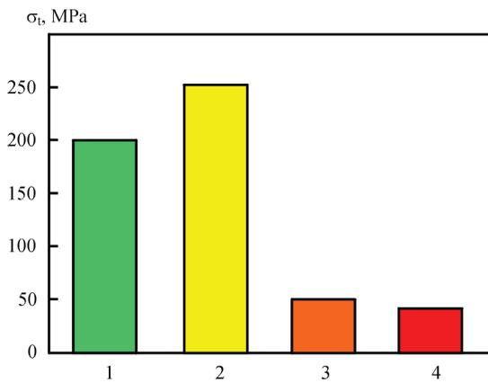
**Figure 6.** Strength of brazed Cu–W joints: in the initial state after brazing (1); after neutron irradiation in the SM-2 reactor at  $T = 100$  °C and a dose of  $5 \cdot 10^{21}$  neutron/cm<sup>2</sup> (2); at  $T = 310$  °C, in the SM-2 reactor, dose of  $5 \cdot 10^{21}$  neutron/cm<sup>2</sup> (3); in the BOR-60 reactor at  $T = 400$  °C, dose of  $5 \cdot 10^{22}$  neutrons/cm<sup>2</sup> (4)
