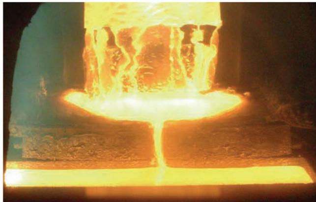
Producing 165x950x2500 mm slab-ingot of PT-3V titanium alloy
