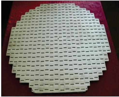
**Figure 1.** General view of brazen antenna array
