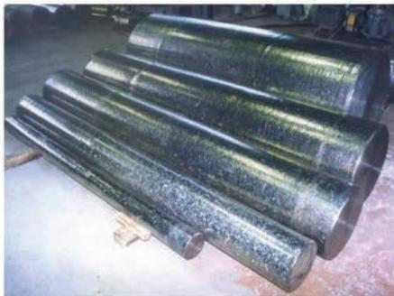
Titanium ingots of 100–600 mm diameter
