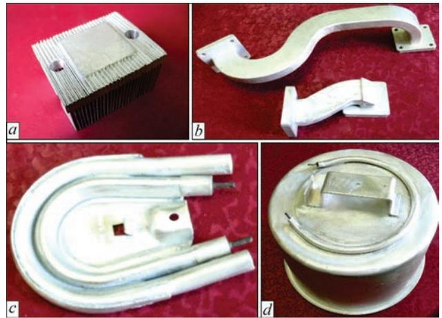
**Figure 3.** Brazen products of aluminium alloys: *a* — plate aluminium heat exchanger; *b* — element of ultra-high frequency module; *c* — tubular heating elements for household appliances (*d*)
