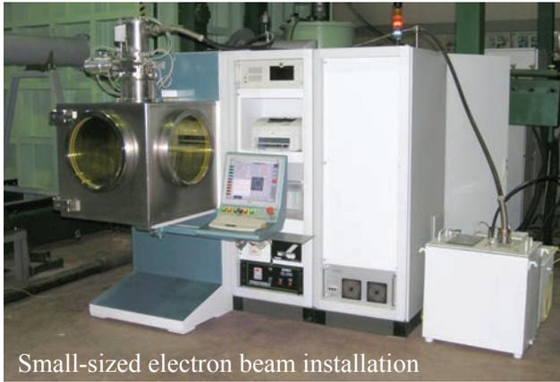
Small-sized electron beam installation
