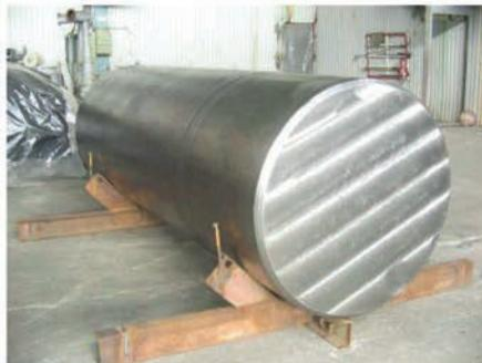
Titanium ingot of 1100 mm diameter
