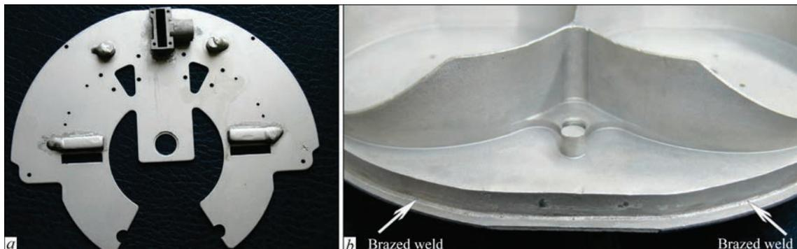
**Figure 2.** Appearance of thin-walled aluminium waveguide (*a*), brazen weld along the perimeter of the structure (*b*)
