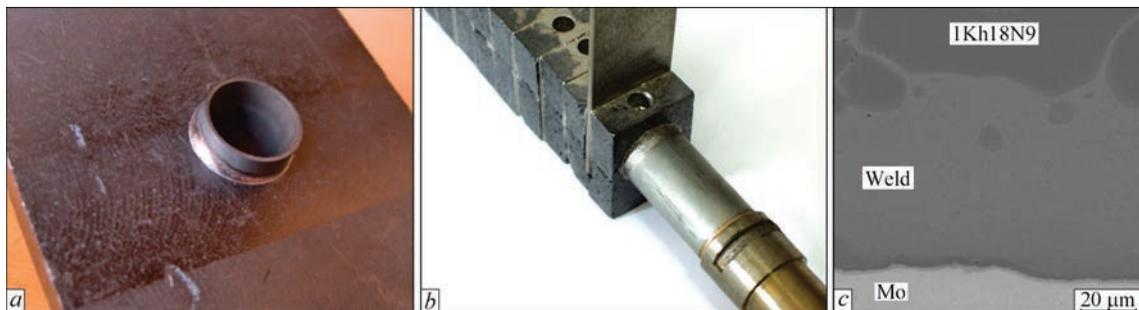
**Figure 7.** Brazed assembly graphite–molybdenum (*a*) and model of diverter device (*b*) containing brazed elements Mo–C (stainless steel) produced by vacuum high-temperature brazing for thermocyclic tests; microstructure of brazed joint molybdenum–stainless steel (*c*)
