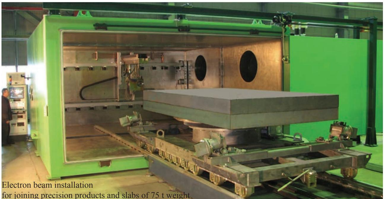
Electron beam installation for joining precision products and slabs of 75 t weight
