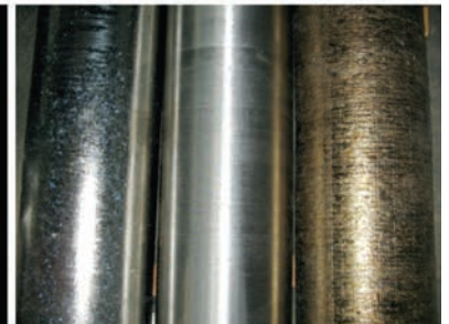
Titanium ingot surface: surface-melted; machined; cast
