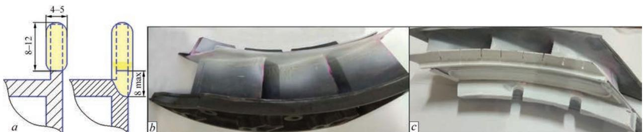
**Figure 2.** Characteristics of the required cross-section of the deposited bead at restoration of HPT SNB side sealing element from ZhS6K alloy (a) and appearance of its surface restored by multilayer MPPS after liquid-penetrant testing (b, c)
