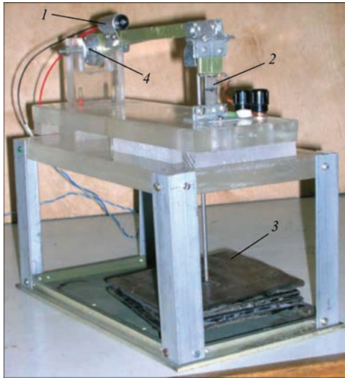
Figure 1. Laboratory welding unit: 1 — laser sensor of electrode movement; 2 — electrodes; 3 — weights; 4 — lever axis
