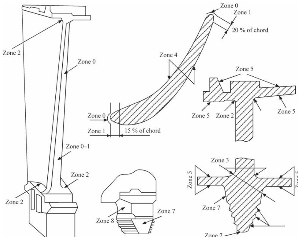
**Figure 2.** Scheme of working uncooled blade with a single-crystal structure of CM96-BI alloy
