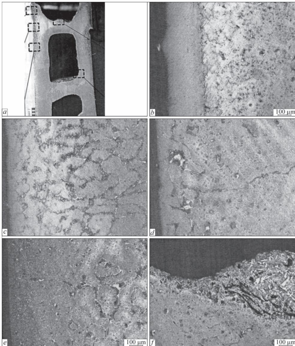
**Figure 3.** Macrosection of the blade (*a*), microstructure with corrected surface defects (*b*, *c*, *d*), base metal (*e*) and brazed sign hole (*f*)
