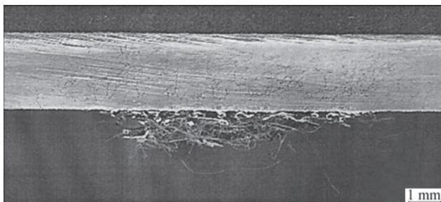
**Figure 4.** Macrostructure of the blade metal in the area of surface defect correction with a protective coating layer
