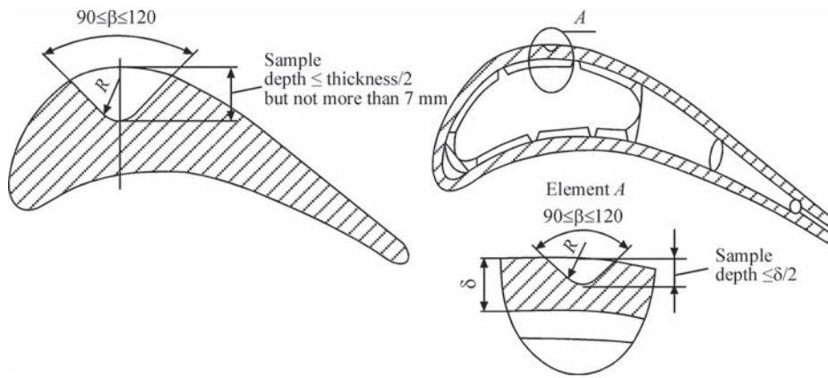
**Figure 1.** Development of surface defect such as cavity of the blade with a polycrystalline structure of CM93-BI alloy
