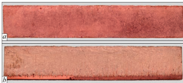
Figure 5. Formation of weld metal in the longitudinal section along the axis of M1 copper with 100 mm length during EBW in the flat position along the butt ( \times 1.5 ): a — without an insert; b — with an insert with VT1-00 thickness \delta = 0.05 mm. EBW conditions: U_{acc} = 60 kV, I_b = 197 mA; v_w = 7.5 mm/s; \Delta I_f = 5 mA; l_w = 200 mm; D = 1.5 mm
