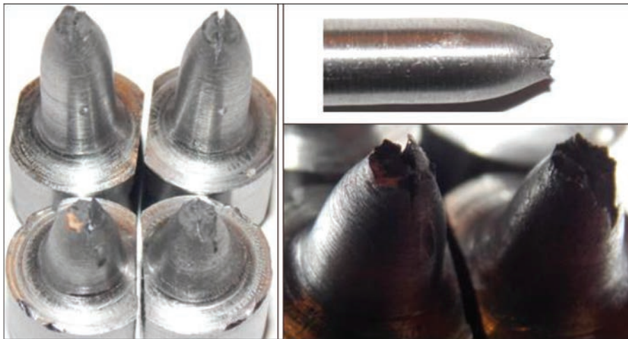
Figure 5. Delamination in the fracture of samples at tensile testing of longitudinal welded joints
