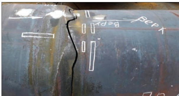
Figure 1. Fragment of the dismantled pipe with fracture region and marks for cutting out templates for investigations and mechanical testing
