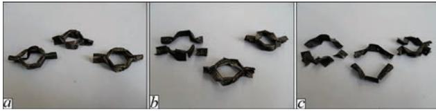
**Figure 7.** General view of samples of individual honeycombs after annealing and mechanical compression testing,  $T_{\text{an}}$ , °C;  $t_{\text{an}}$ , min: a — 600, 150; b — 600, 600; c — 600, 1200
