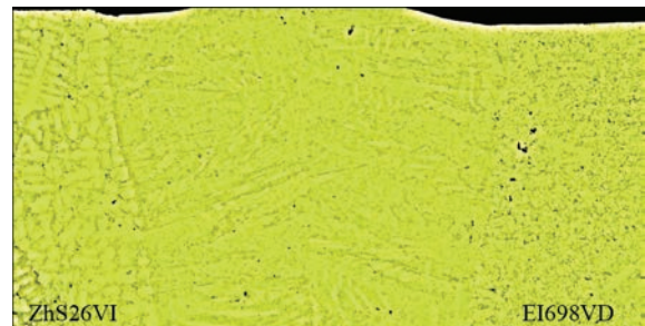
Figure 7. Welded joint of ZhS26VI with EI698VD alloys (maximum content of EI698 alloy components) ( \times 50 )
